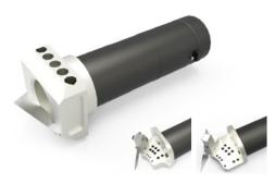
A dedicated tool used for corrugated and sandwich materials to make V groove, can change blade slope (0°, 15°, 22.5°, 30°, 45°) to achieve different results.
